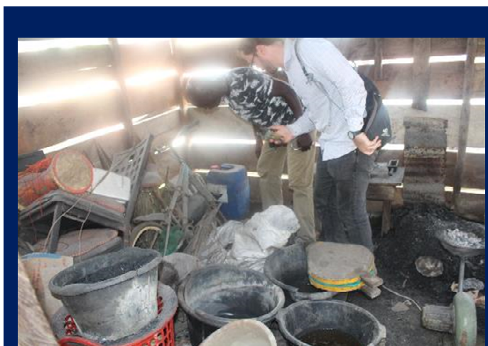
Figure 4: Observing an artisanal gold refinery in a market in Asankrangwa. The gold is heated with a coal fire (right); the blue jerry can contained sulphuric acid.
