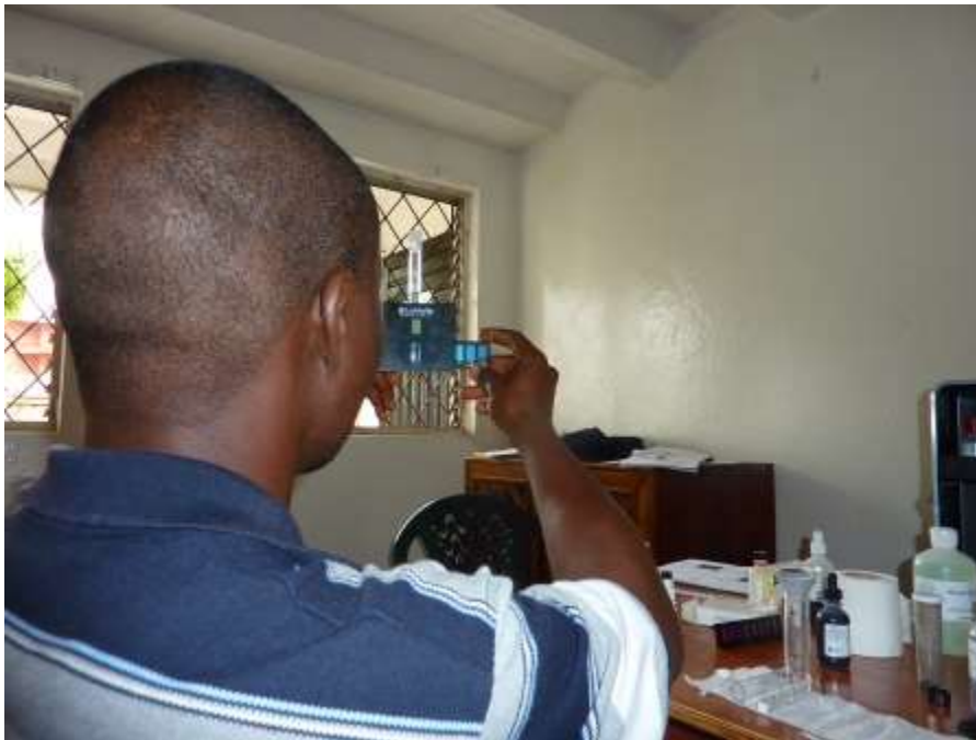
Color change used to measure soil phosphate with the LaMotte kit.
