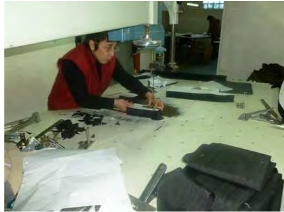
Workers operate cutting equipment without safety gloves.
